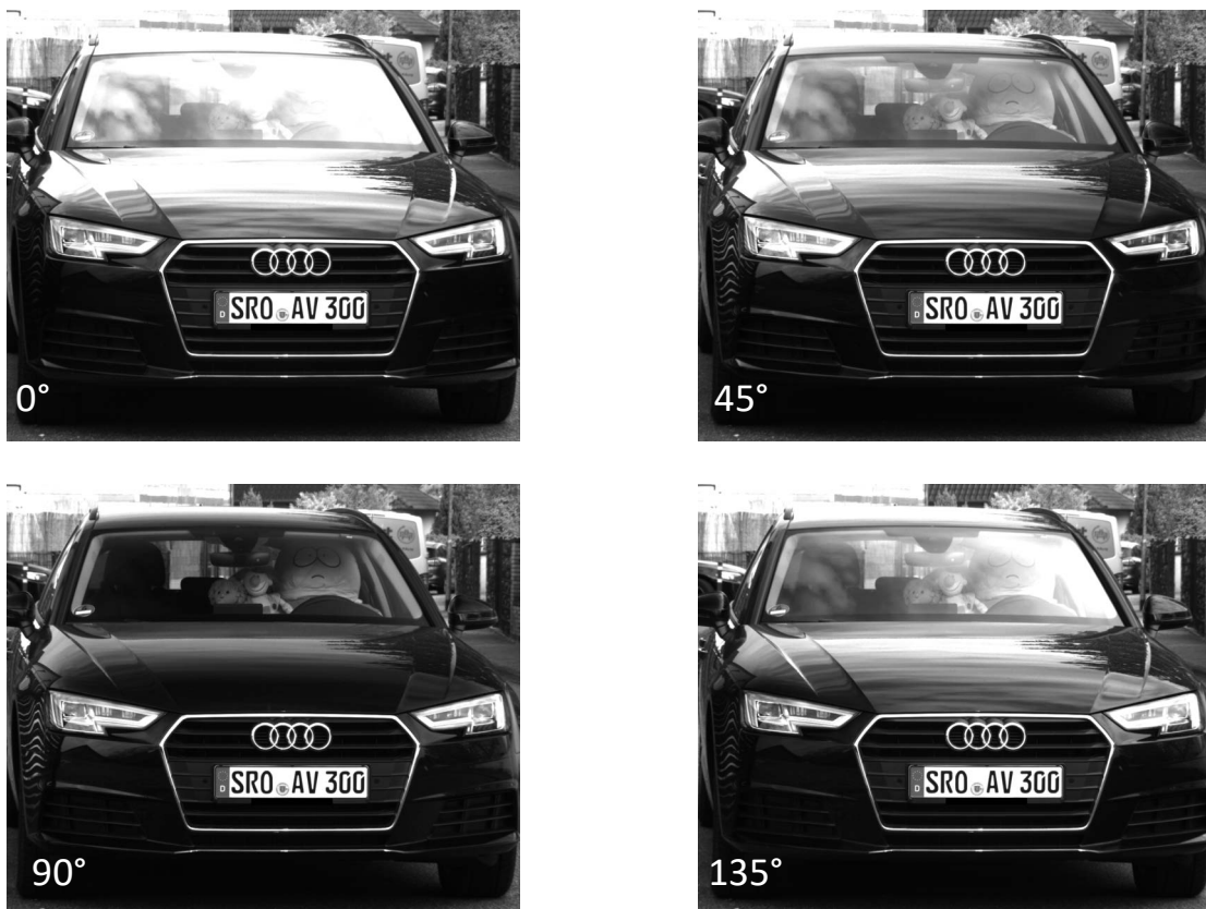
Figure 5: Polarization angle versus image brightness in sub-images
